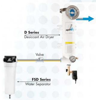
It is also possible to dry the air directly at the point-of-use (ex: paint booth, dust collector, sand blast cabinet, etc.). In this case we need to dry the air in two stages: the separation of the water using an Air / Water Separator, followed by a SUPER-DRY desiccant air dryer.
